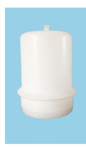
ZCK-H Filter cartridge with a polypropylene cage, uses encapsulated technology. No adhesives or glue are used in the manufacturing process, and all bonding is done by thermal welding. The inner core uses multiple winding filters to increase the filtration area and speed up the flow rate. The precision range can be 20~300um. The filter can be applied to the solution with high viscosity of filter material liquid.
