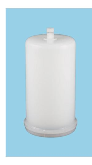
ZCK-H Filter cartridge with a polypropylene cage, uses encapsulated technology. No adhesives or glue are used in the manufacturing process, and all bonding is done by thermal welding. The inner filter is pleated, which has the effect of deep filtering. The precision range can be  $50\sim300$ um. The filter can be applied to the solution with high viscosity of filter material liquid.
